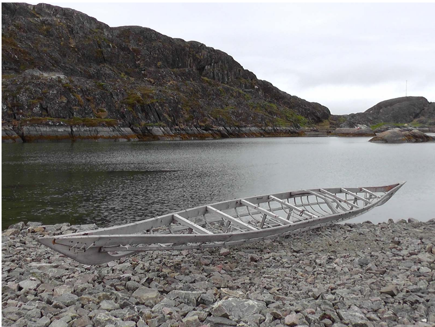
11One of the "dead" qajaqs outside the Sisimiut Clubhouse. It only needs a new fabric skin and a paaq / manhole, and it's ready for duty - after all these forgotten years.
